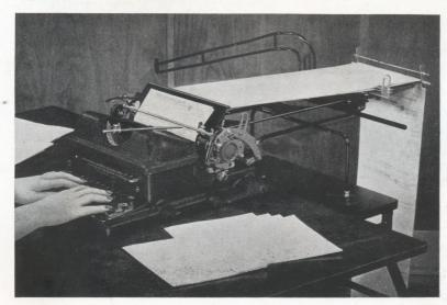
The Electric Forms-Writing Machine brings an accuracy and new speed to the preparation of important business documents. Every mechanical operation of this machine is completely electrical—the entire keyboard including tabulator, back spacer, space bar, shift key and carriage return. All types of forms, even up to 20 carbon copies, are written with speed and ease.
